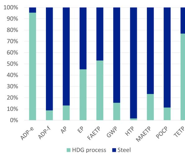
Figure 5. Contribution of the environmental impacts of steel production and the HDG process (HDG plant 1 in 2016)
