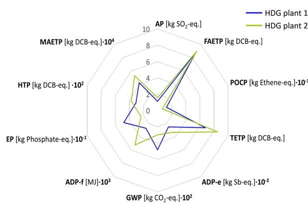
Figure 7. Environmental impacts of HDG plant #1 and HDG plant #2, in 2016
