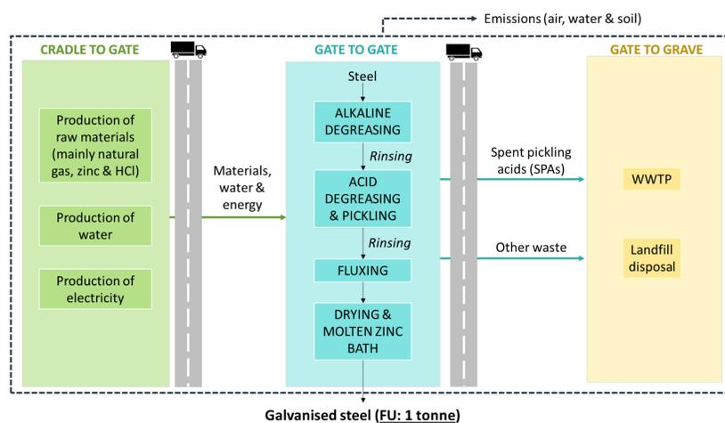
Figure 3. System description of the cradle to grave analysis of the HDG process
