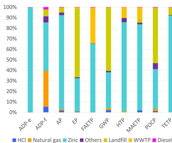
Figure 6. Main environmental impacts during the cradle to gate and gate to grave life cycle (HDG plant 1 in 2016)
