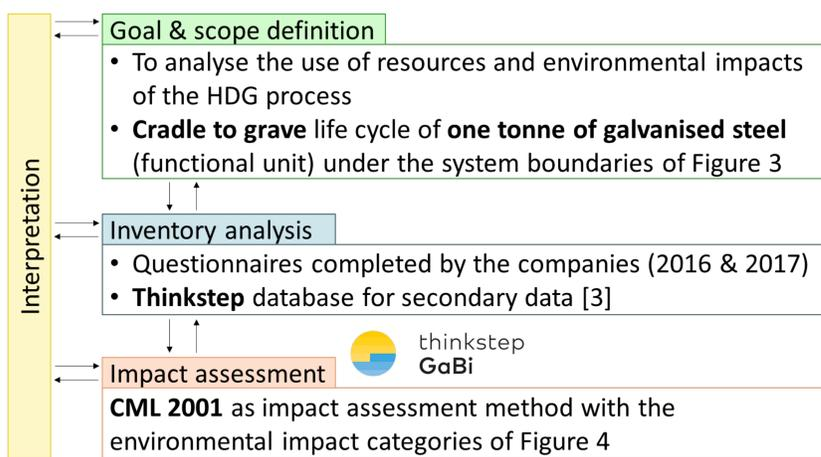
Figure 2. LCA stages [1, 2]
